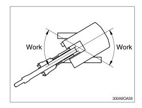
Conversely, if thrust is excessive or breaking is performed with boom of the lower chassis raised as shown, the machine may suddenly tip toward the movement. The breaker body may strike the broken rocks violently resulting in damage.
